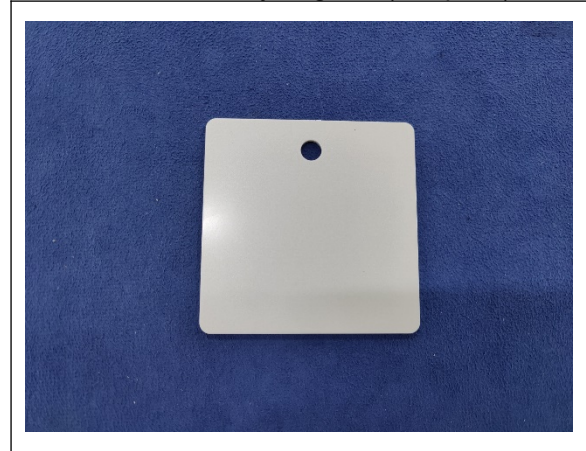
After soap and cleaner effects test (sample 2)
