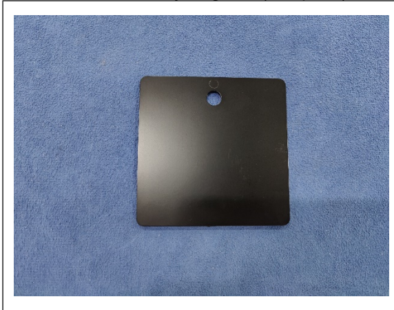
After soap and cleaner effects test (sample 1)
