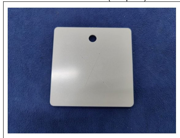
After adhesion test (sample 2)
