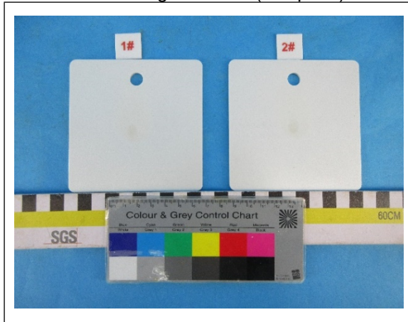
After falling sand test (sample 2)
