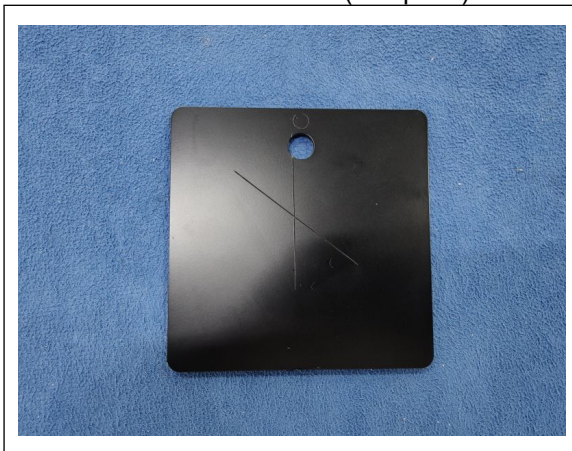
After adhesion test (sample 1)
